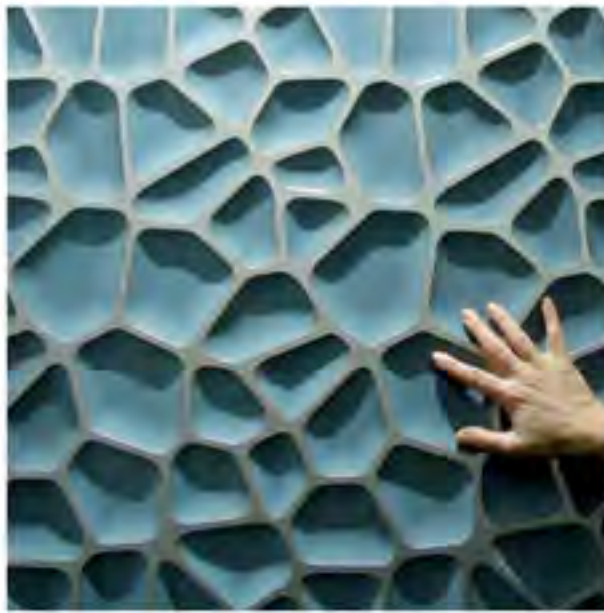
PVT Blue colored MDF / brushed aluminum overlay. PD: 0.25". PT: 0.75". Pattern Type: Repeating. Pattern repeats every 12" along the 4' side of panel and every 24" along the 8' side of panel.
