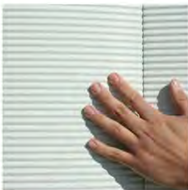
W12B Shown in finish by others. Profile Depth: 0.156". Overall pattern depth: 1". PT: 1.5". Pattern Type: Repeating. It is limited to 4'x8' or 4'x10' panels only.
