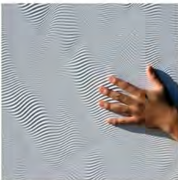
COP 011 Snow White membrane finish. PD: 0.2". PT: .75". Pattern Type: Continuous. Standard panel size is 48" x 96". Pattern is NON-repeating. Panel layout must be submitted in order to achieve panel match. Pattern direction may be selected in vertical direction or horizontal direction.
