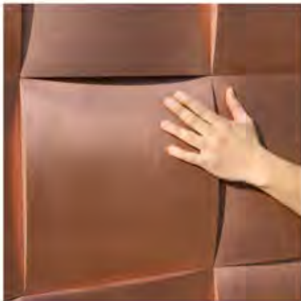
PLW12 Shown in copper metallic paint. PD: 1.5". PT: 2". Pattern Type: Repeating. Thickness includes 0.5" Baltic Birch plywood backer. It is limited to either 4'x8' or 4'x10' panel sizes only.
