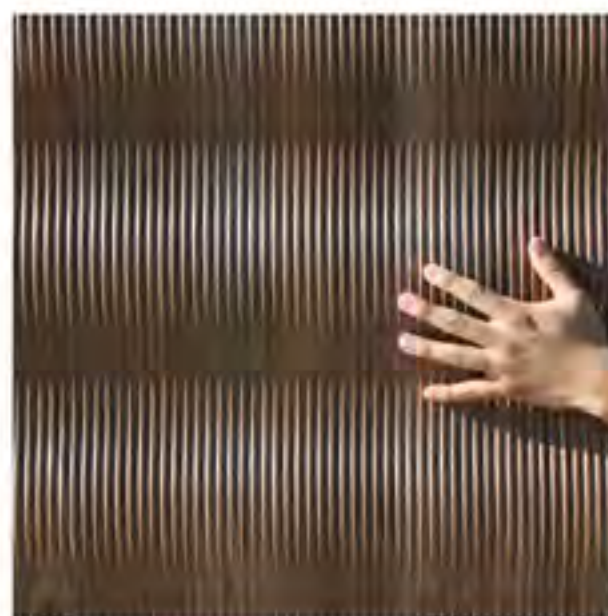
W406B Shown in Amati PC membrane finish. Profile depth: 0.156". Overall pattern depth: 1". PT: 1.5". Pattern Type: Repeating. It is limited to 4'x8' panels only.
