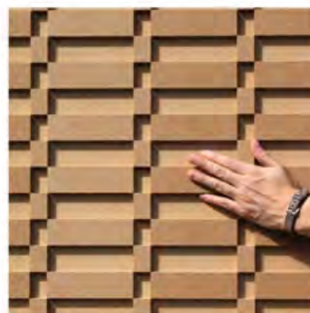
CB 15-5-1 Shown in unfinished IDF* PD: 0.375". PT: 1.5". Pattern Type: Repeating. Rectangle sizes are 1.5" x 5" and 1.5" x 1". It is limited to 4'x8' panel only. * - if product is ordered raw IDF then the overall thickness will be 1.25 inches.
