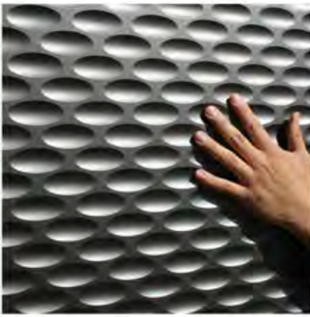
POP006 Shown in finish by others. PD: 0.17". PT: 0.75". Pattern type: Repeating/ Continuous. Notes: Pattern repeats every 12 inches perpendicular to pattern direction. Pattern direction may be selected in vertical direction or horizontal direction.
