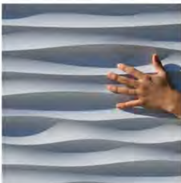
SOT002x4 Shown in white paint finish. PD: 1.2". PT: 1.5" Pattern Type: Repeating/ Continuous. Notes: Pattern repeats every 48 inches perpendicular to pattern direction and every 96 inches parallel to pattern direction. Must be "A-B" panel match for horizontal repeat.
