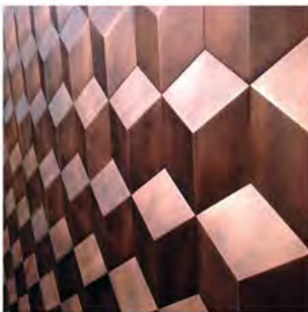
Bizarro Shown in Antique Copper. Nominal Panel Size: 51" x 96" Pattern Depth: up to 0.75". Panel Thickness: 0.75" plus 0.5". Pattern Type: Stacked. Each piece is connected to a backer-board of 0.5" baltic birch plywood using the Interlink system.
